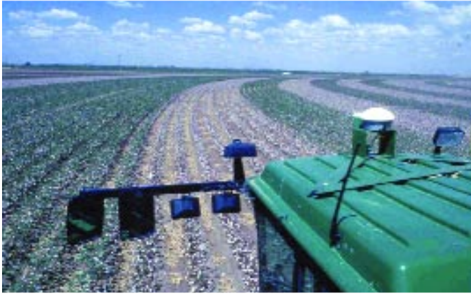
White-capped GPS unit mounted on top of harvester.
